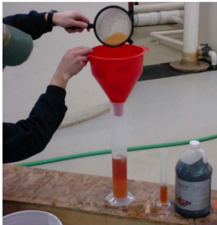
Fig. 10. Total volume of eggs is being determined by displacement.
