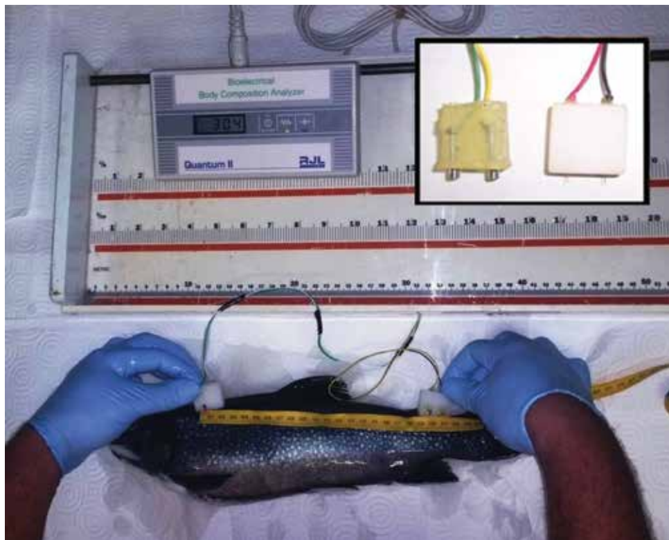
Figure 1. The BIA analyzer consists of a solid state instrument (here, RJL Systems Quantum II) with two pairs of signal and detection electrodes. Electrodes (inset) are often needle electrodes that penetrate just below the skin of the fish. Rod electrodes, which measure along the surface of the skin, are shown for comparison (from Hafs 2011), but these surface electrodes are more likely to have contact issues, particularly for scaled fishes. Photo credit: K.J. Hartman.
