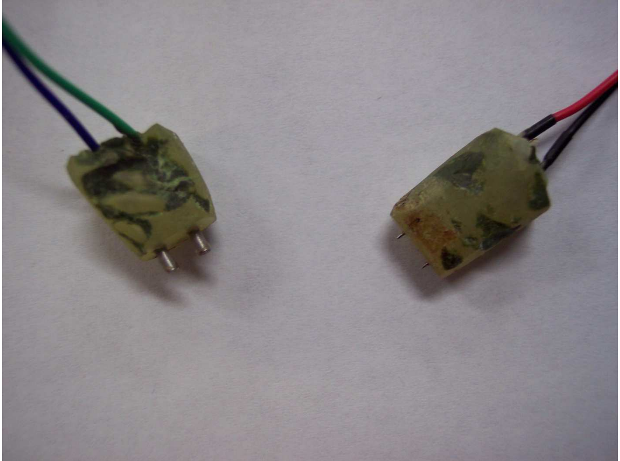
Figure 1.–Picture of external rods (left) and subdermal needle (right) electrodes used in this study.
